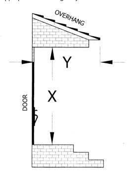
X = distance from bottom of door to base of overhang
